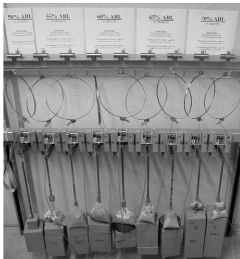
Figure 2. Experimental set-up for CCT tests
