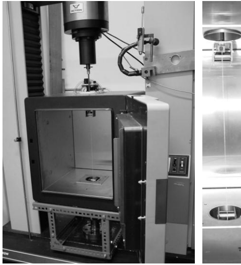
Figure 1. Experimental set-up for tensile and SIM tests
