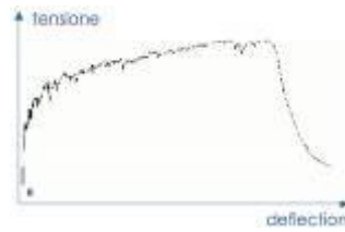
Figure 4: flexural behaviour of the mortar HFE-tec SHCC1
