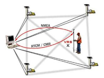
Figure 3 The VRS measurement process
