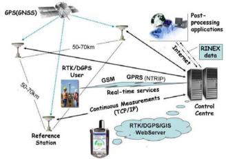
Figure 2 Basic functional components and services to be provided by HEPOS
