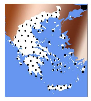
Figure 1 Schematic coverage of the stations comprising the HEPOS network
